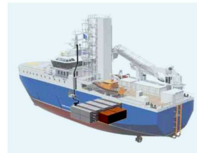
Figure 7 - Battery vessel configuration
